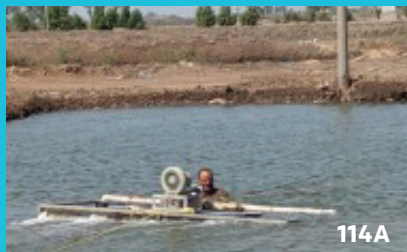
Figure 114A & B. WhiteWater Units connected to the IPRS cells and in the open pond. Solid wastes were collected two or three times daily by manually vacuuming from the QZ. Waste was pumped to waste settling tank at pond bank.
