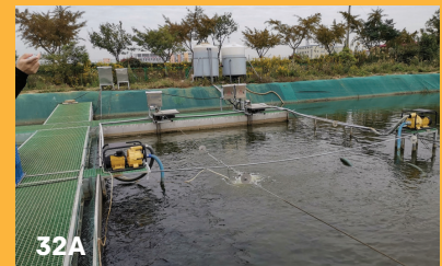
Figure 32A & B. Two types of waste collection systems cables and rails
