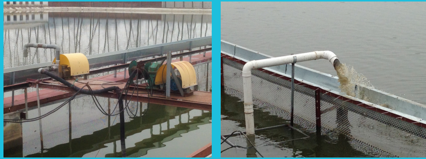
Figure 70. Rail mounted solid waste pumping system that pumps water to sloped trough
